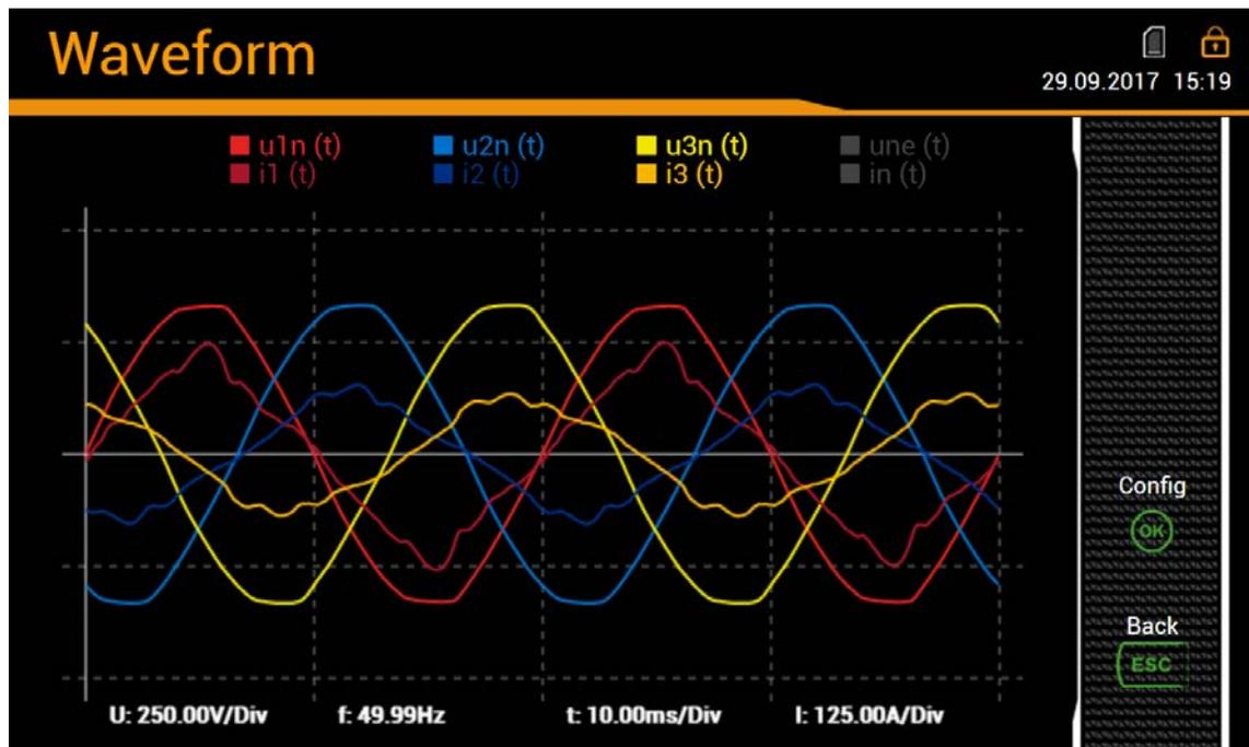
Current and voltage curve in the main power supply of a Swiss electronics producer
