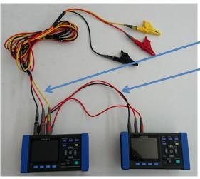
CLAMP ON POWER LOGGER PW3360
