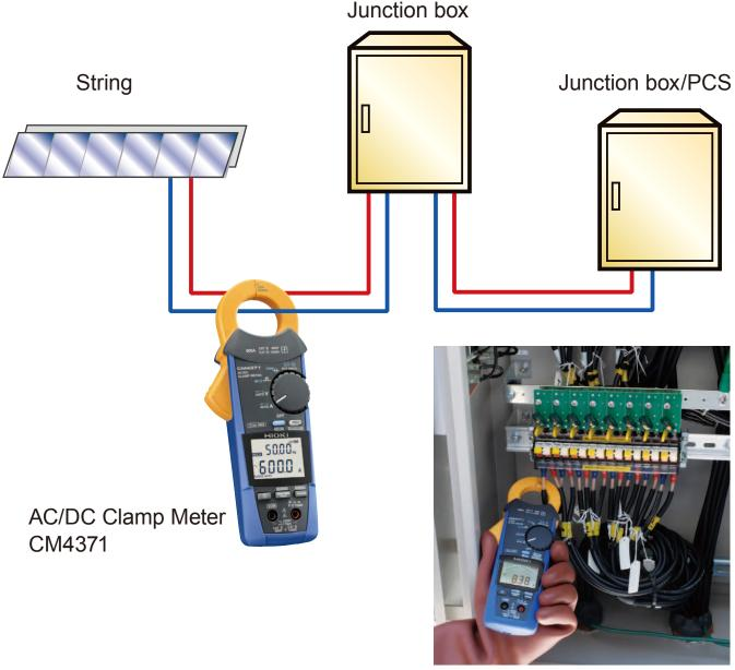
Be sure to clamp in the correct direction according to polarity.
